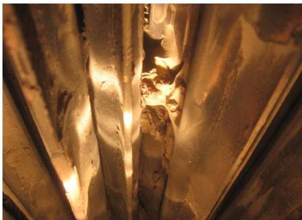
Case 4: The economiser headers are in the flue path. The economiser tubes are finned type and also staggered. The clearances were so less that the ash could easily trap in to narrow spacing of the tubes. Clogged ash formed during a fouling coal had led to erosion within the bank. Placing headers inside had also led to higher apparent gas velocity.
